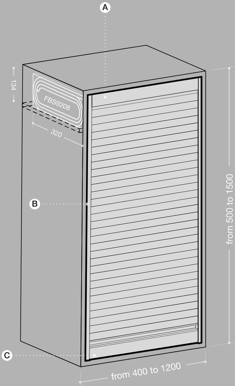
misure in mm - dimensions in mm
