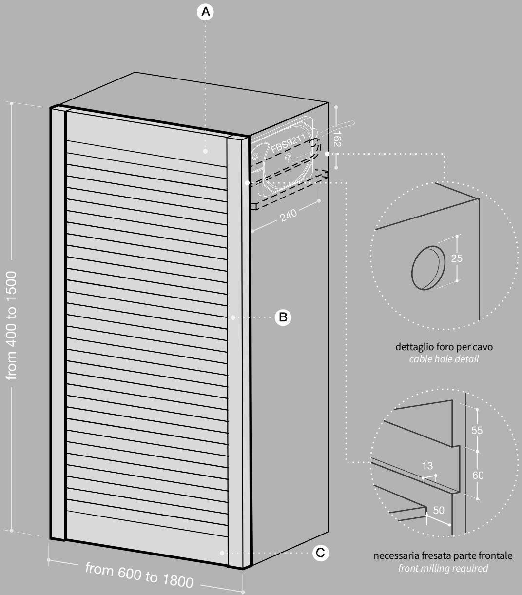
misure in mm - dimensions in mm
