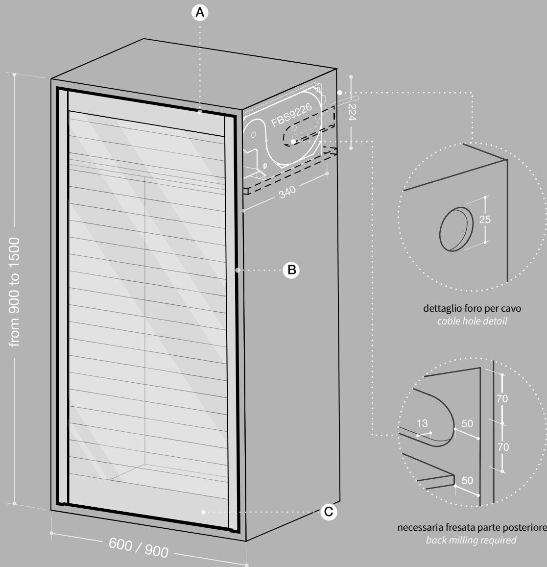
misure in mm - dimensions in mm
