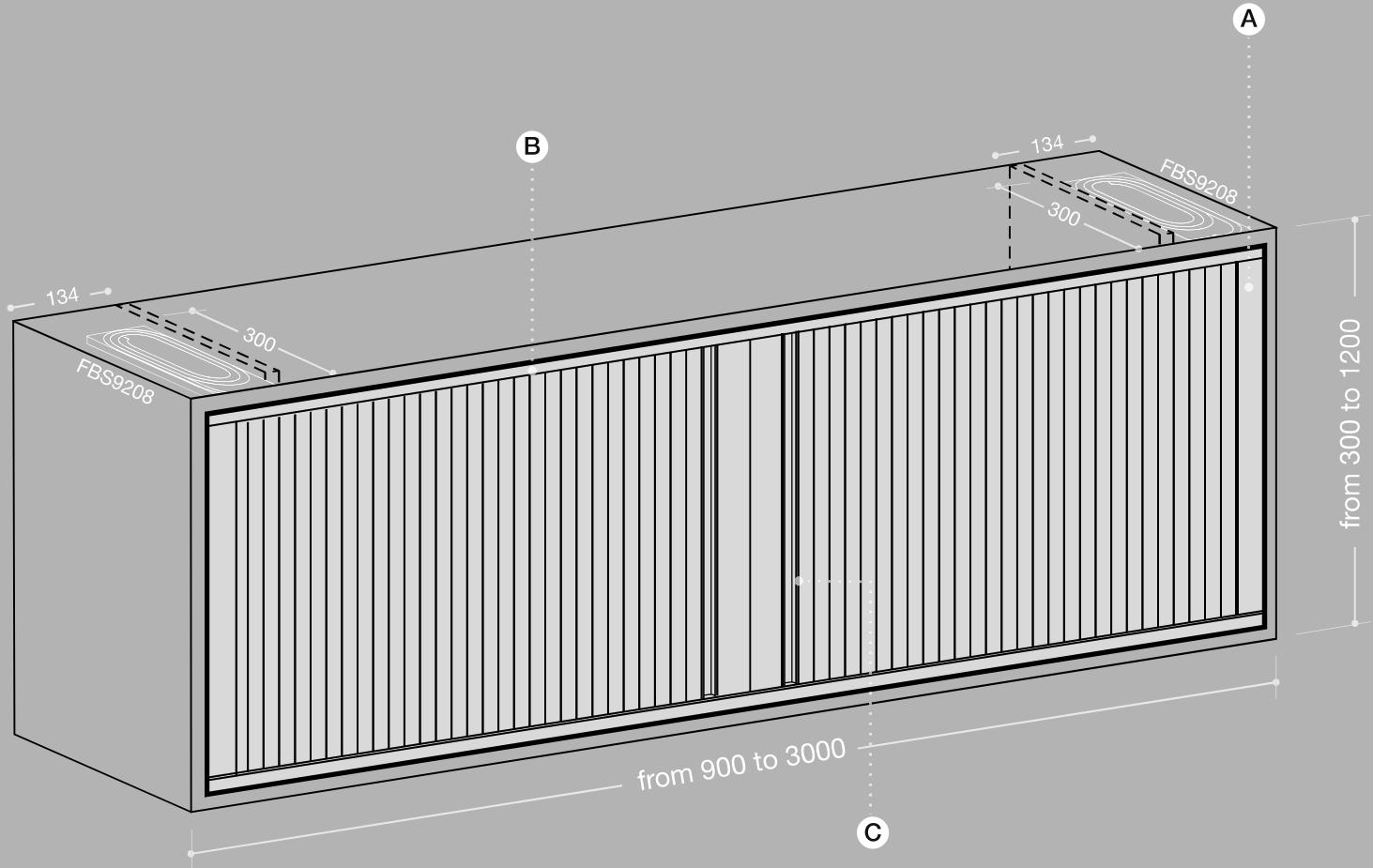
misure in mm - dimensions in mm
