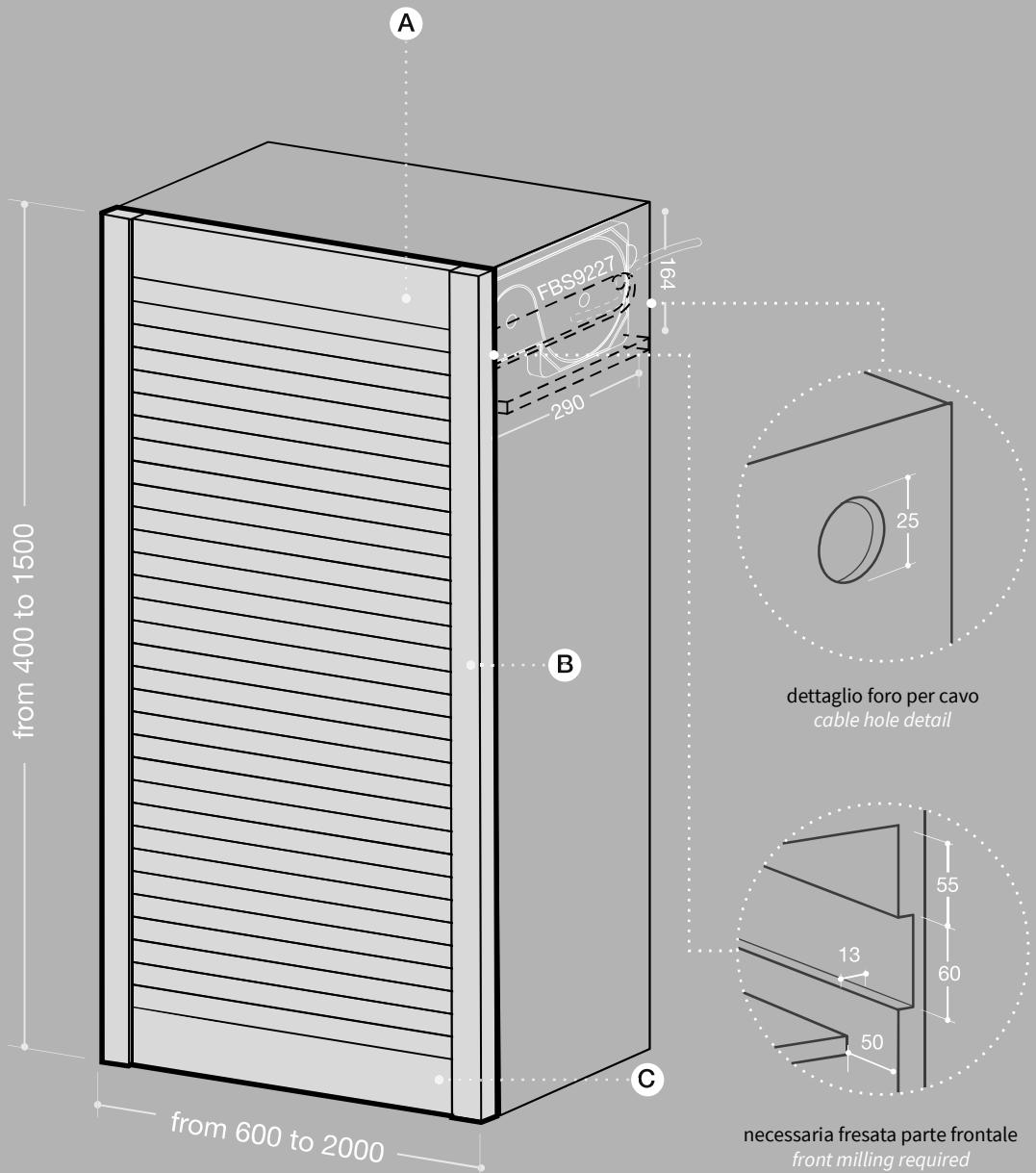
misure in mm - dimensions in mm
