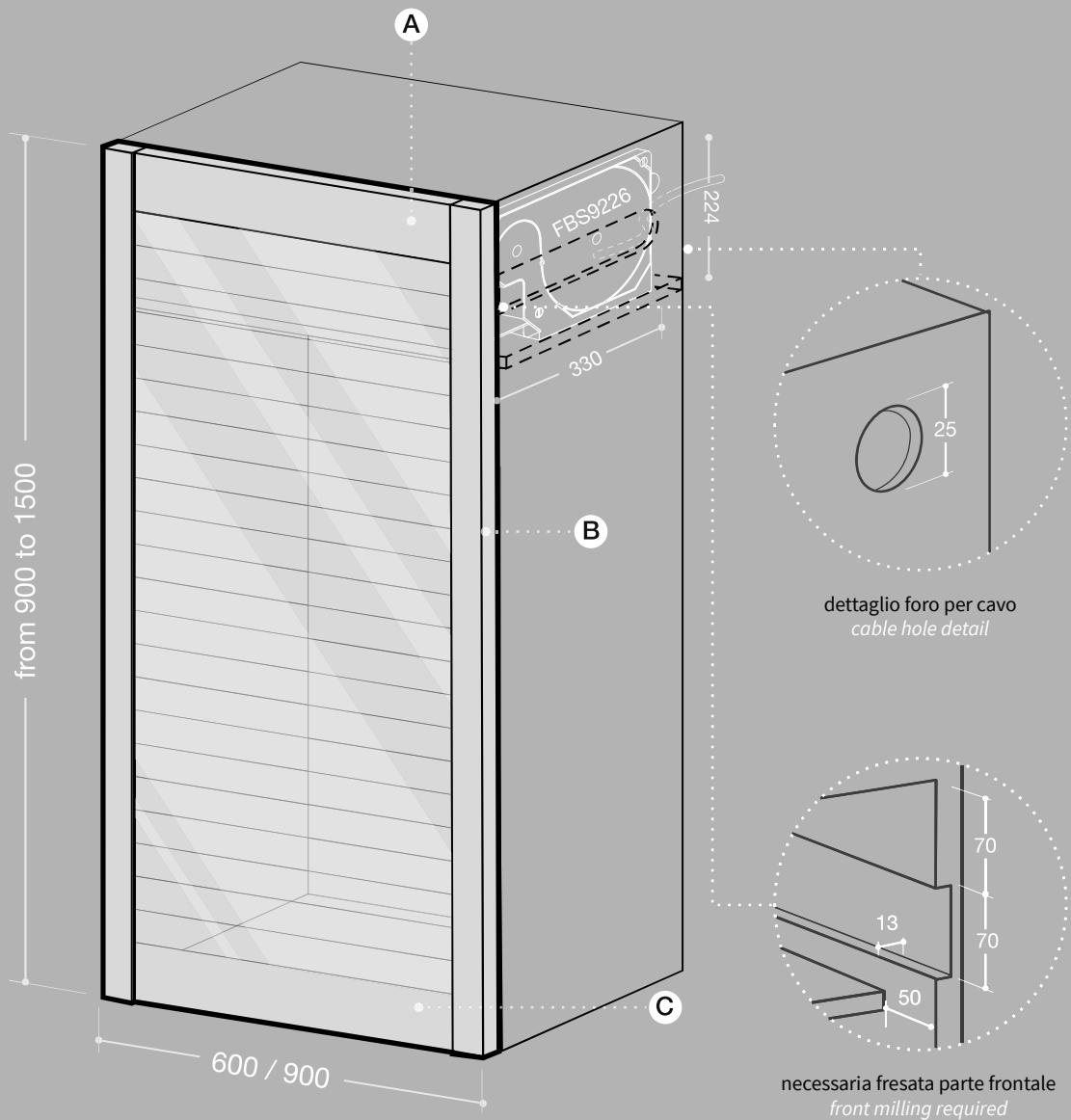
misure in mm - dimensions in mm
