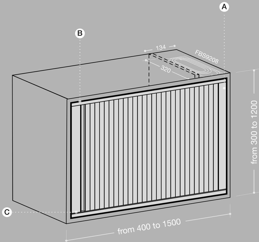
misure in mm - dimensions in mm
