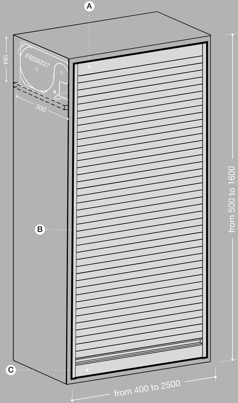
misure in mm - dimensions in mm
